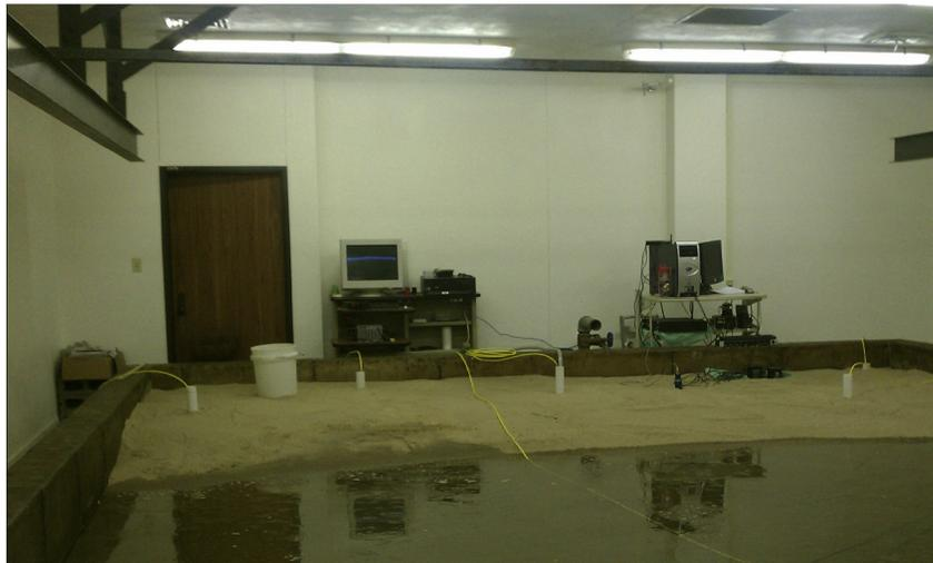
Fig. 2. Sand tank experiment site with five wells, seismic source and accelerometers.
