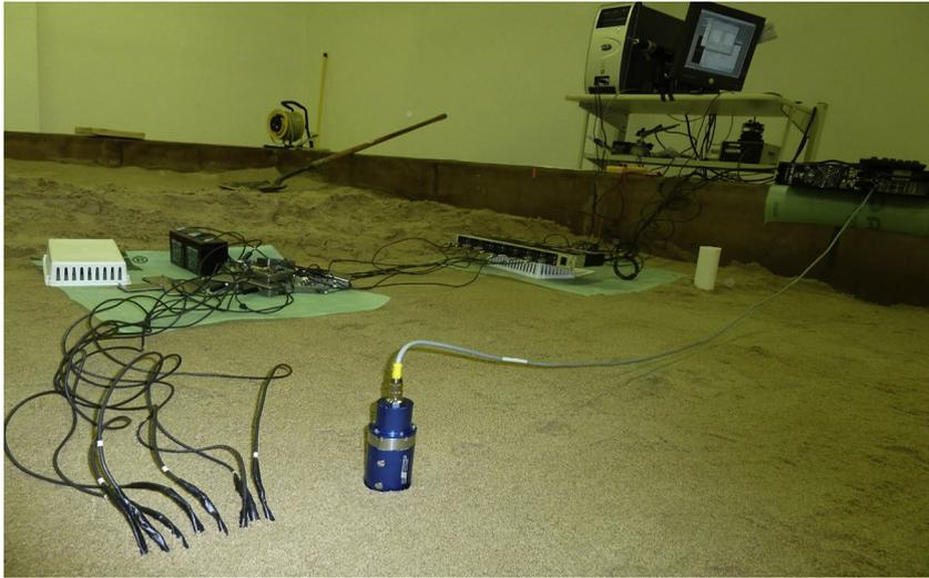
Fig. 3. Seismic source and accelerometers.
