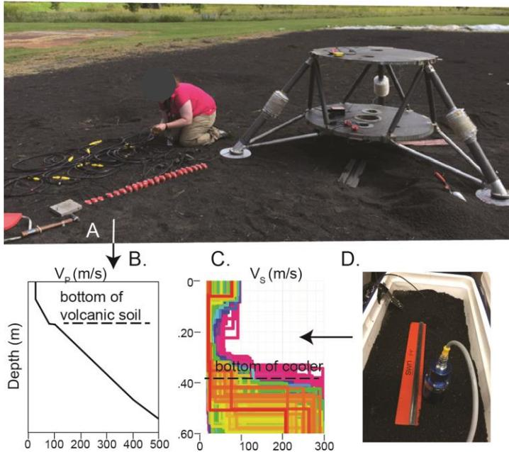
**Figure 1. Marshall Space Flight Center Regolith Field geophone seismic experiment adjacent to mock lunar lander; Summer 2019 B. Velocity model derived from refracted seismic arrivals C. A range of seismic inversion results and their RMS misfits (0 .14 --red,to 0.27-- blue) against a dispersion curve D. Smaller-scale experiment in the same soil. Signal from a magnetostriictively seismic source (blue) is collected with buried wired sensors (kHz). Ruler is 30 cm. long.**
