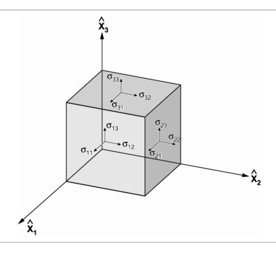
Each face of the cube can experience traction or stress. Stress on a surface can be treated as a "stress vector" and is also called a **traction vector** ( $\vec{T}$ ), where, in the limit, traction equals force per unit area at a point on one face:
