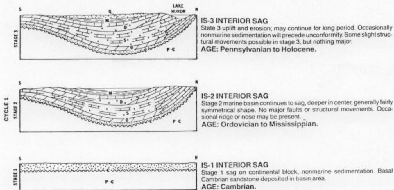
FIG. 3—Evolution of interior sag basin illustrated by restored cross sections in three stages. Example from Michigan basin.
