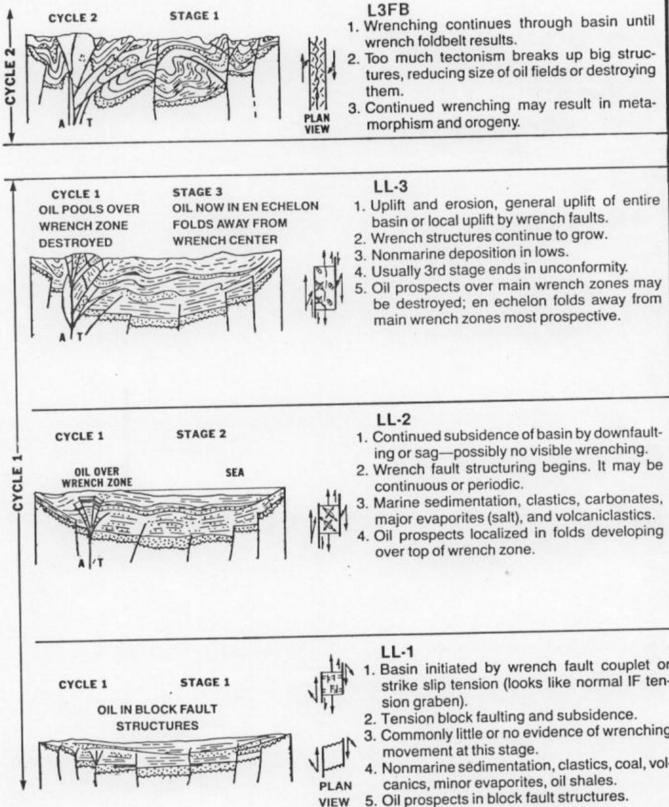
FIG. 8—Evolution of wrench or shear basins. LL = lateral. Development of convergent plate wrench in three stages (LL-3, 2, 1). L3FB shows final step in many wrench basins, that of foldbelt caused by wrenching. This is final step in process that creates basin and finally destroys it. After initiation of basin (LL-1), movement may cease in any succeeding stage. Basin may also stop strike-slip mode and change to polyhistory basin.
