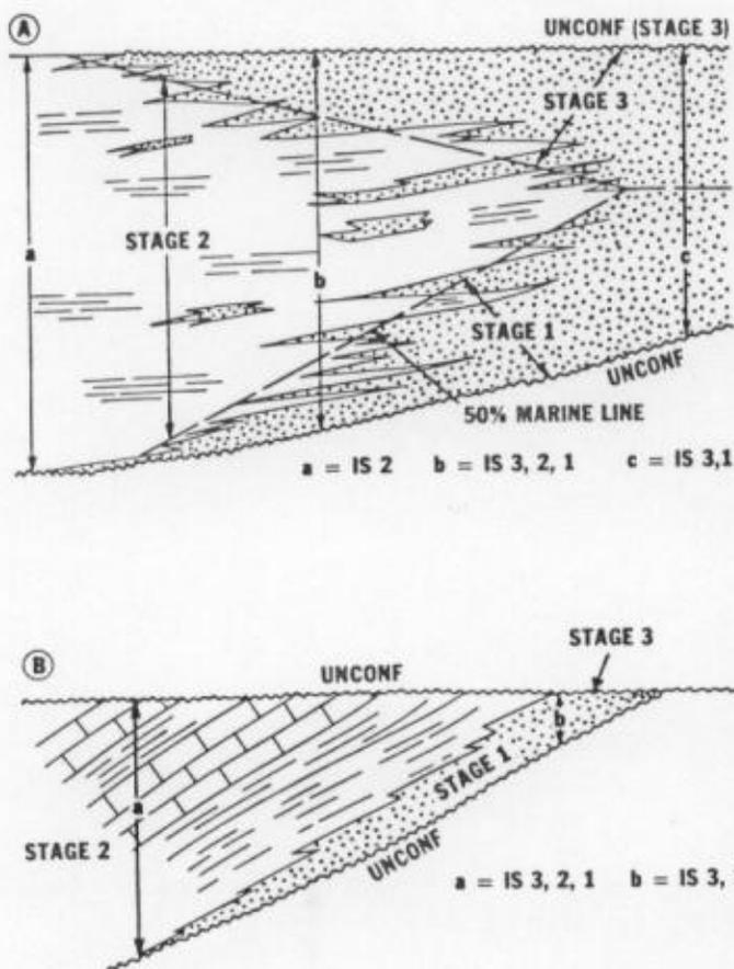
FIG. 2—Relation of stages to sedimentary wedges. (A) Sedimentary wedge showing transgressive wedge base (stage 1), wedge middle (stage 2), and regressive wedge top plus unconformity (stage 3). Dashed median line separates stages. (B) Sedimentary wedge where unconformity has cut out stage 3 and part of stage 2.
