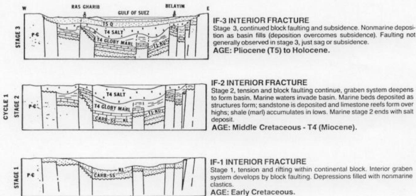
FIG. 4—Evolution of interior fracture basin illustrated by restored cross sections in three stages from Early Cretaceous to Holocene. Example from Gulf of Suez.
