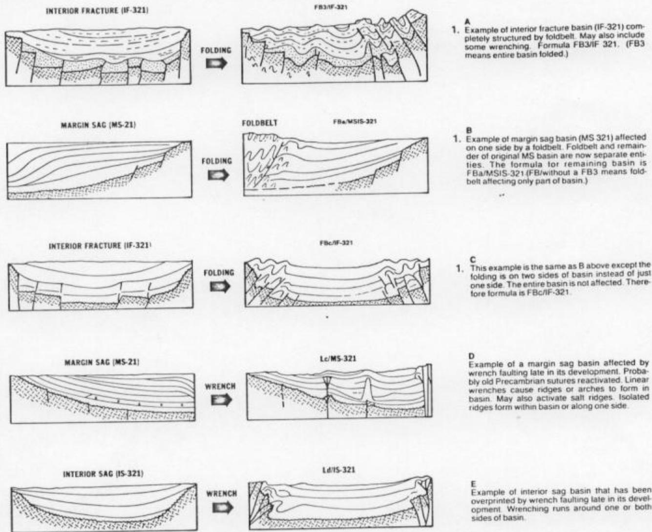
FIG. 12—Examples of polyhistory basins, showing simple divergent basins overprinted by foldbelt and wrenching tectonics.
