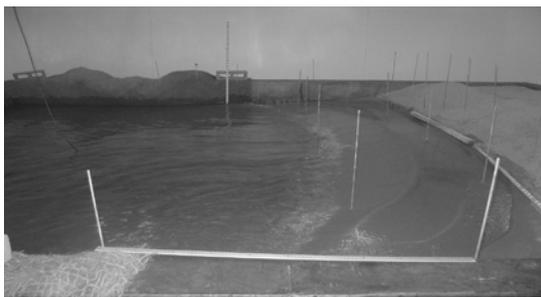
**Figure 1.** Louisiana State University seismic physical modeling sand tank (Figure 1)
