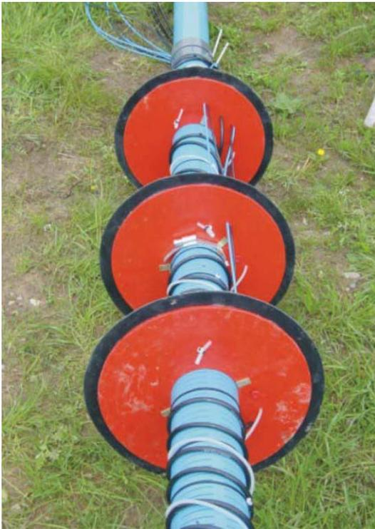
Fig. 8. Multilevel sampler for large diameter pumping wells.
