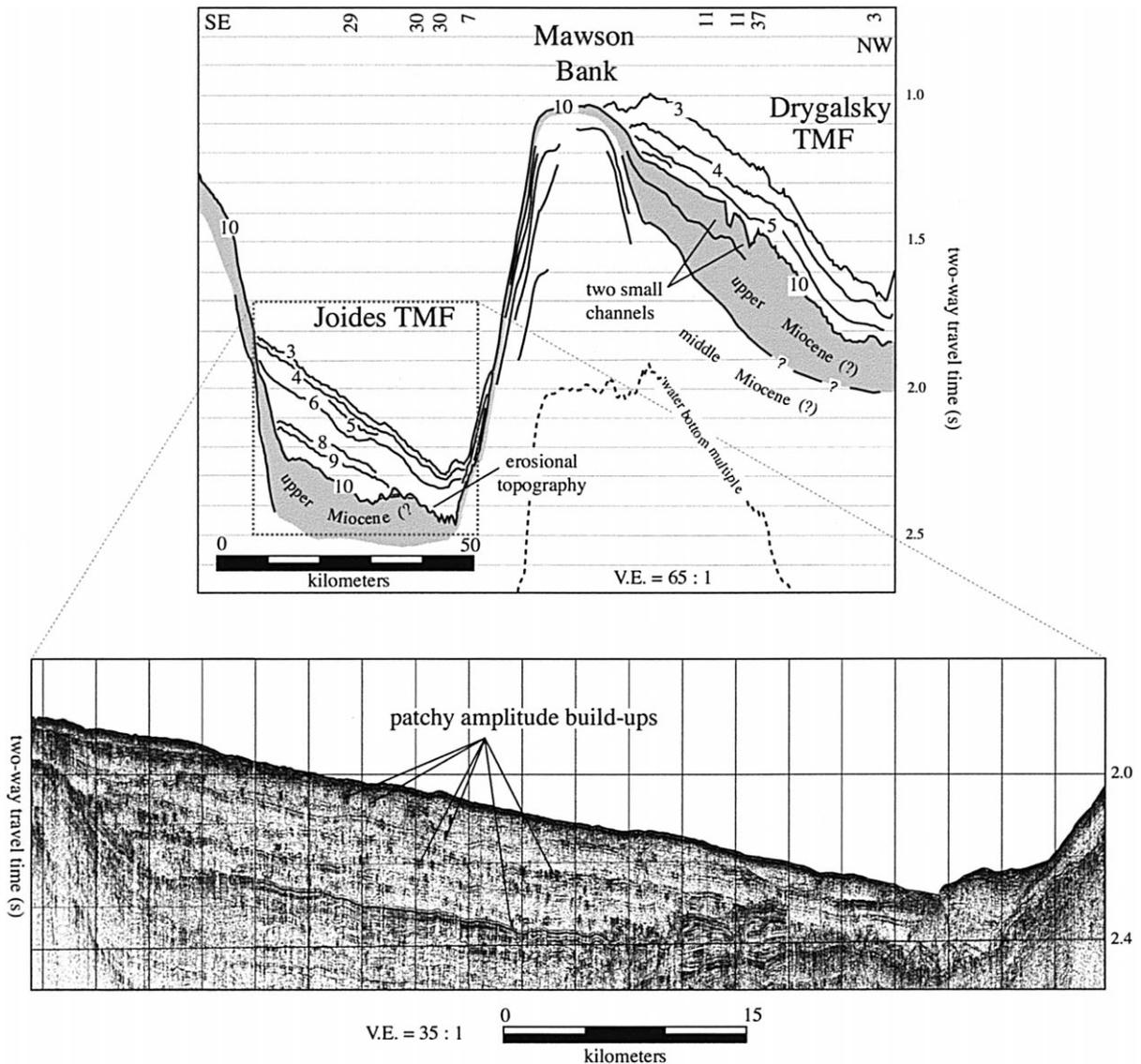
Fig. 7. Line drawing and uninterpreted seismic segment of strike-oriented Profile 2 on the upper slope beyond the mouths of Joides and Drygalsky basins. Unconformity 10 has erosional morphology at the axis of the Joides Slope Basin and at two small channels on the eastern flank of the Drygalsky Basin. See Fig. 1 for location.
