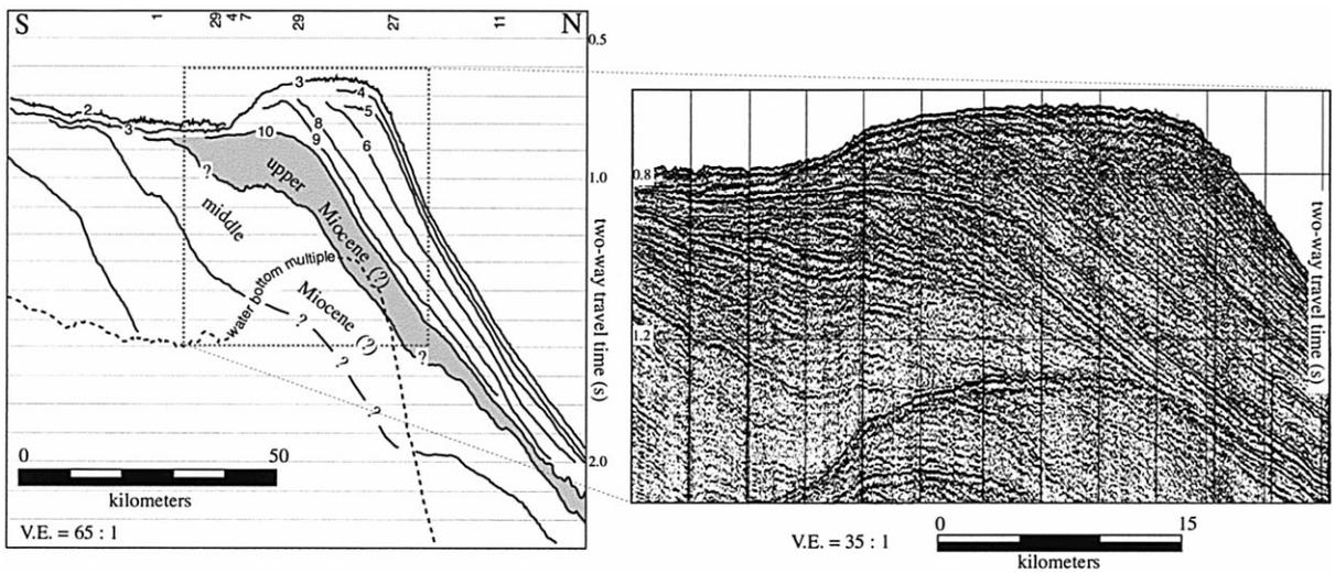
Fig. 6. Line drawing and uninterpreted seismic segment of dip-oriented Profile 39 crossing from the mouth of Joides Basin to the Joides Slope Basin. This profile shows a thick wedge of prograding-slope strata at the mouth of Joides Basin. Unconformities 4, 5, 6, 8, 9 and 10 are truncated at Unconformity 3. See Fig. 1 for location.
