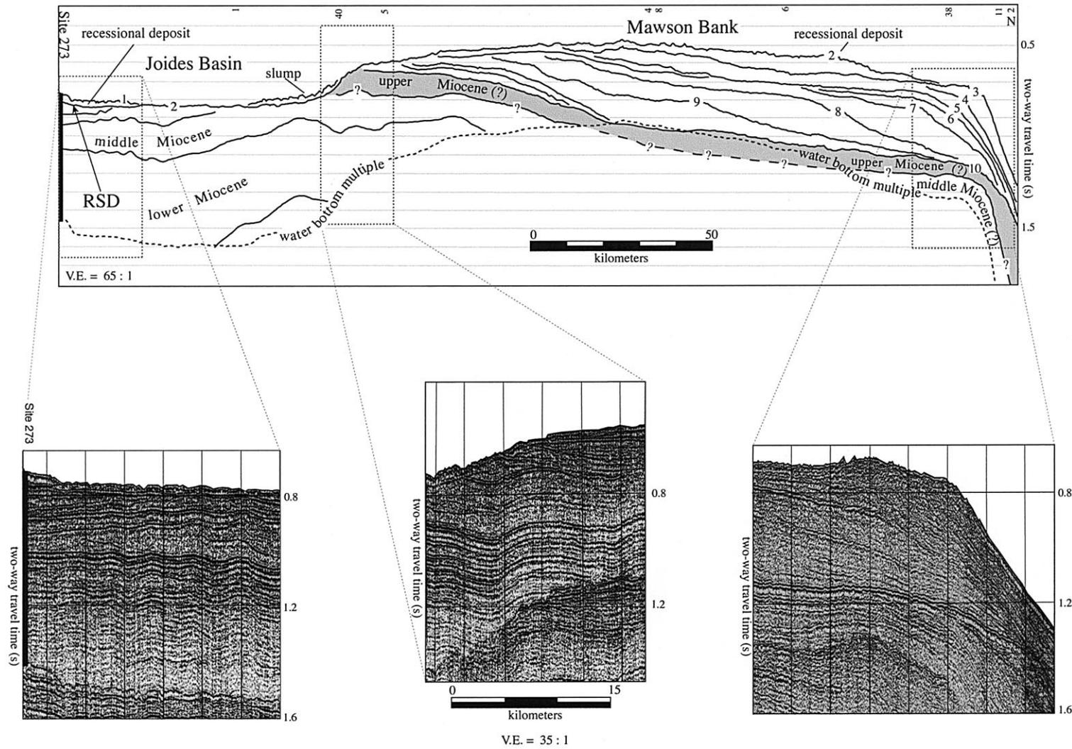
Fig. 2. Regional line drawing and uninterpreted seismic segments of dip-oriented Profile 37. At Site 273, the strata above the Ross Sea Discontinuity (RSD) are Pliocene–Pleistocene in age and correspond to Unit 1. See Fig. 1 for location.
