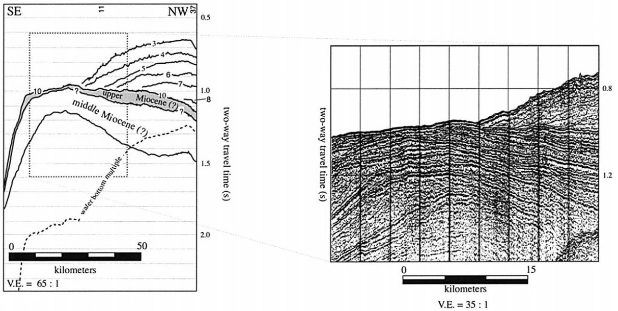
Fig. 5. Line drawing and uninterpreted seismic segment of Profile 38 which crosses the Mawson Bank outer shelf and the western flank of the Joides Slope Basin. The stratigraphic patterns indicate to us that during the Unconformity 10 grounding-event, the ice sheet expanded to the shelf edge whereas subsequent expansions did not prograde this segment of the margin. See Fig. 1 for location.
