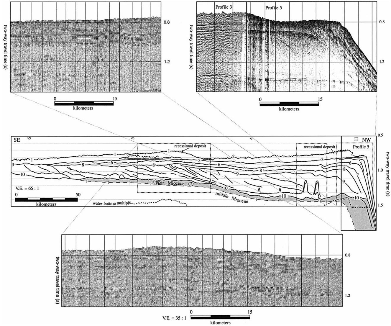
Fig. 4. Regional line drawing and uninterpreted seismic segments of dip-oriented Profile 3 joined to Profile 5 on the shelf at Drygalsky Basin. The line drawing shows the stratigraphic relationship between the deep axis of the Unconformity 10 paleo-trough and the overlying strata. Downlap and outbuilding occurred during the deposition of the upper part of Unit 9–3. Units 1 and 2 exhibit a backstepping pattern on the shelf.
