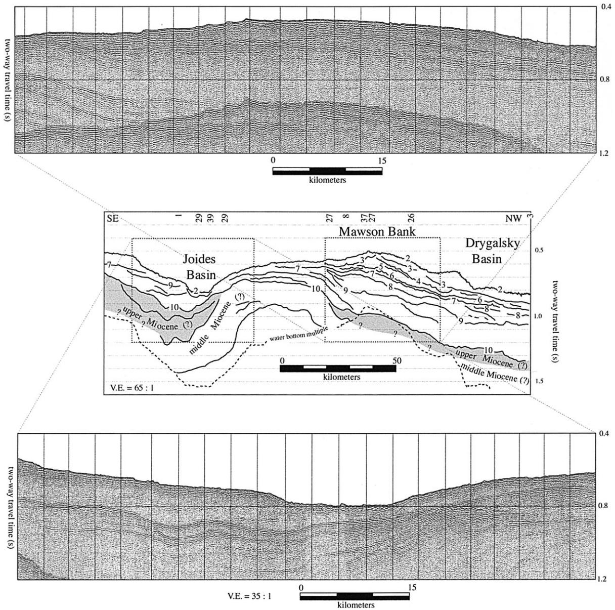
Fig. 3. Regional line-drawing and uninterpreted seismic segments of strike-oriented Profile 4 along the outer shelf extending from Joides Basin to Drygalsky Basin. A paleo-bank and two paleo-troughs at Unconformity 10 are roughly coincident with Mawson Bank, and Joides and Drygalsky basins. See Fig. 1 for location.
