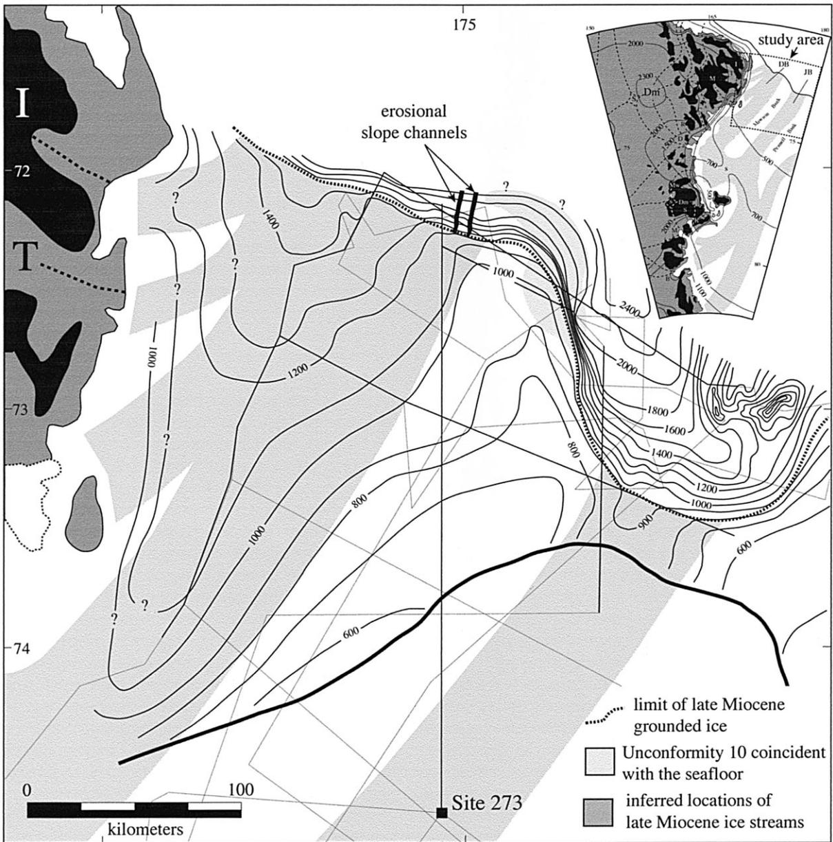
Fig. 8. Time–structure contour map at Unconformity 10. Contours are in two-way travel time below sea level. The dashed line shows the seaward extent of topset truncation of the underlying strata. The heavy solid line indicates the landward limit of Unconformity 10. The light-shaded area on the outer shelf and upper slope correspond to the area where Unconformity 10 coincides with the seafloor. The inset shows our inference on the location of late Miocene ice streams emanating from the TAM.
