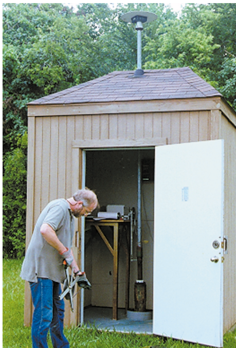
USGS hydrologist measures water levels at an extensometer site, which also serves as a Continuous Operating Reference Station equipped with a GPS antenna and receiver to continuously monitor land subsidence.
