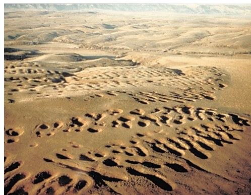
Subsidence pits and troughs formed above the Dietz coal mines near Sheridan, Wyoming. The coal mines were in operation from the 1890s to the 1920s.
