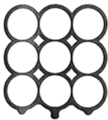
◀ FIGURE 3.9 Pendular water clinging to spheres owing to surface tension. Gravity attraction is pulling the water downward.
