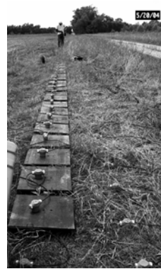
Figure 2: Twenty-three (plus one planted in ground in foreground) 100-Hz vertical component geophones are screwed rigidly to "channel" steel sleds. The heavy weight of each sled (9 kg) assures suitable mechanical coupling with the ground. The line of geophones is oriented west (farthest point) to east. Geophones are placed ~ 0.30 m apart.
