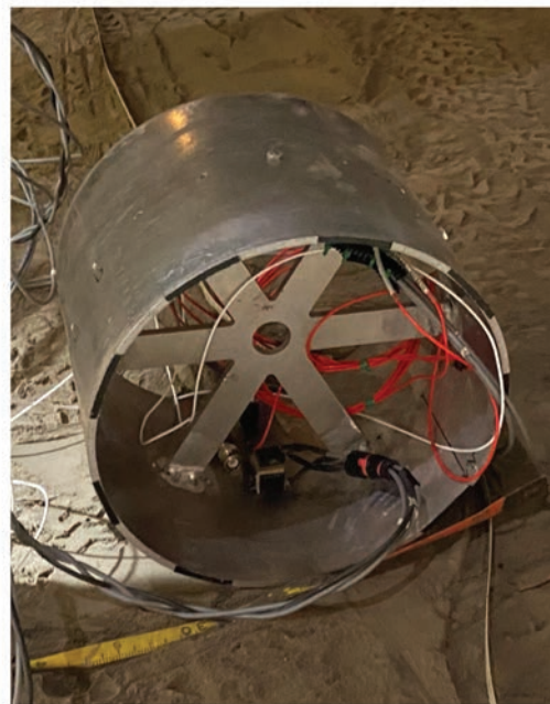
Figure 5. Field deployment of wheel-mounted three-component accelerometer in permafrost loess cave, Alaska. Hammer drop (Table 1) is the source.
