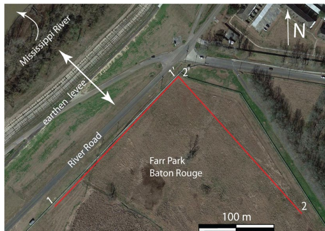
Figure 6. Location of electrical resistivity profiles along two orthogonal lines in the Farr Park study area. Data along both lines were collected on 12.9.20 during a low stage of the Mississippi river (18 ft above sea level) when the ground surface was completely dry and accessible.
