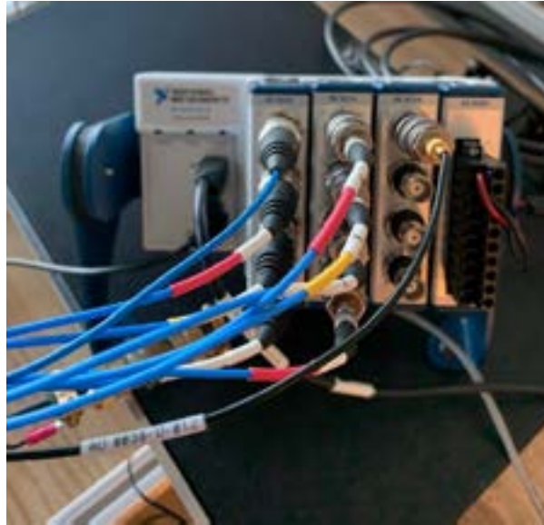
Figure 16. National Instrument DAQ system.
