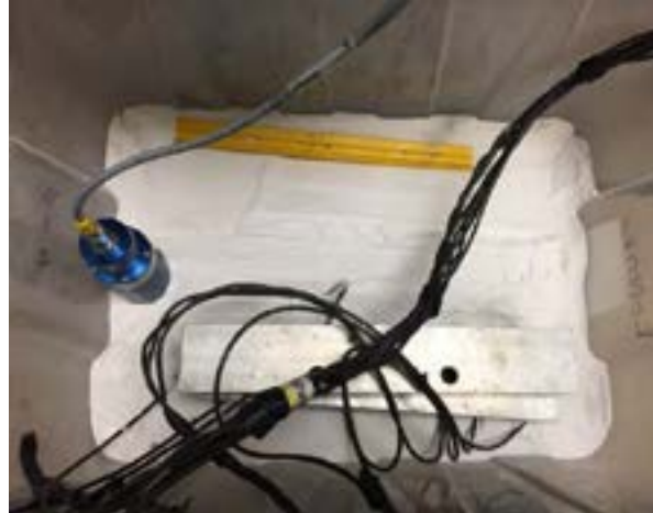
Figure 7. Spatial arrangement of sensor and source for case of ACH-01 sensors. Fixed location of magnetostrictive shaker/vibrator, but ACH-01 sensors are buried 1 cm, and separated 5 cm apart. The first offset between the source and the nearest sensor is 3.8 cm. Grain diameter: < 2^{-4} mm.
