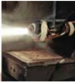
Figure 9. Star 4G Motor During Static Test Firing.
