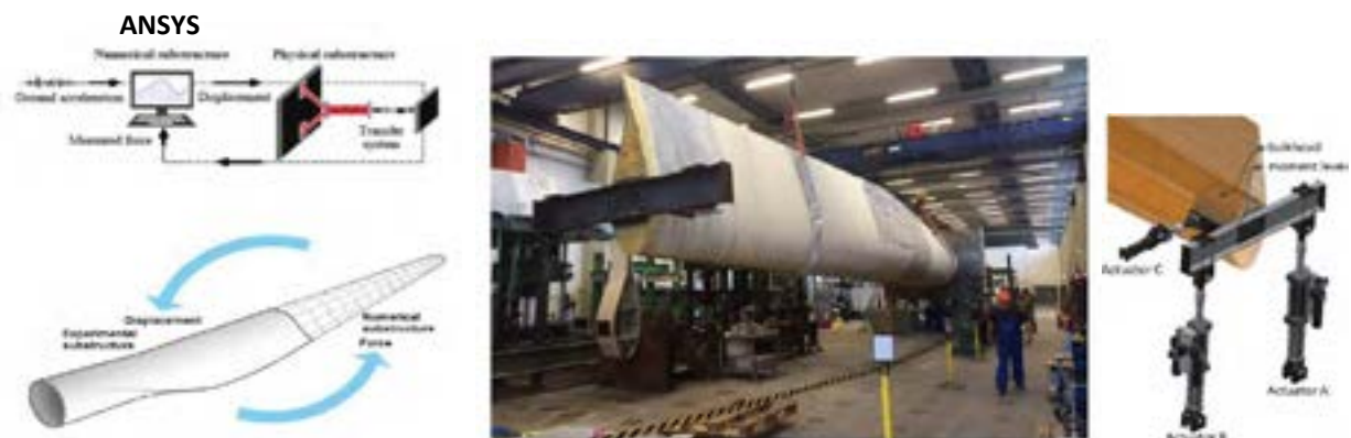
Figure 2. Hybrid Simulation of a blade at Technique University of Denmark [1, 2]
