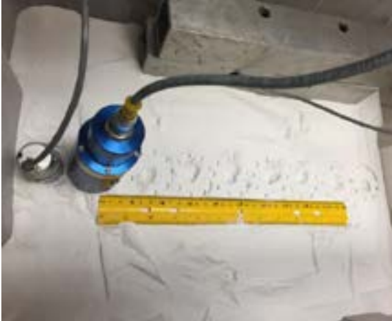
Figure 6. Spatial arrangement of sensor and source for AT23S sensor. Separation between repeated locations of the magnetostrictive shaker/vibrator = 5 cm. The first offset between the source and the nearest sensor is 3.8 cm. Grain diameter: < 2^{-4} mm
