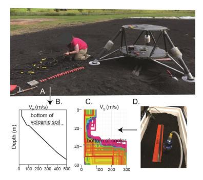
Figure 1. Marshall Space Flight Center Regolith Field geophone seismic experiment adjacent to mock lunar lander; Summer 2019 B. Velocity model derived from refracted seismic arrivals C. A range of seismic inversion results and their RMS misfits (0 .14 --red,to 0.27-blue) against a dispersion curve D. Smaller-scale experiment in the same soil. Signal from a magnetostrictively seismic source (blue) is collected with buried wired sensors (kHz). Ruler is 30 cm. long.
