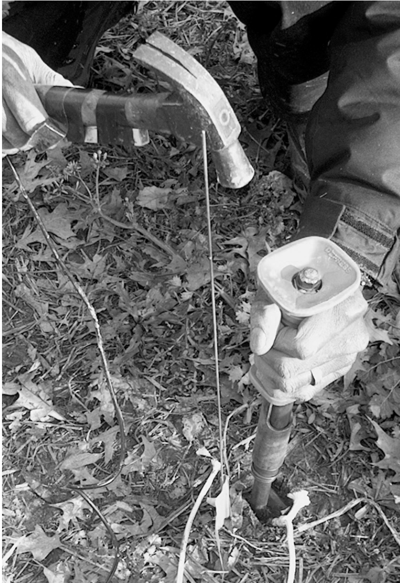
Figure 6-3. PowerHammer (Remington Trademark) 0.22 caliber shell set off by blow from claw hammer. Hammer piston is pushed out and impacts underlying 2-in square steel plate (Case 3). Date: 5/20/04.
