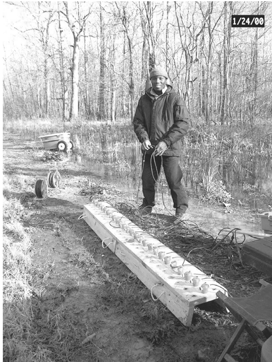
Figure 6-5. Twenty-four 100-Hz vertical geophone sensors are rigidly attached to two four-foot wooden sleds. Each sled weighs approximately 50 lbs. to assure suitable coupling with the ground. The seismic source was a PowerHammer (Remington Trademark) impacting on a 2-in square metal baseplate. LSU graduate student Adeniyi Saanumi is picture above near the first site, adjacent to Core C-1. Date: 1/24/04.
