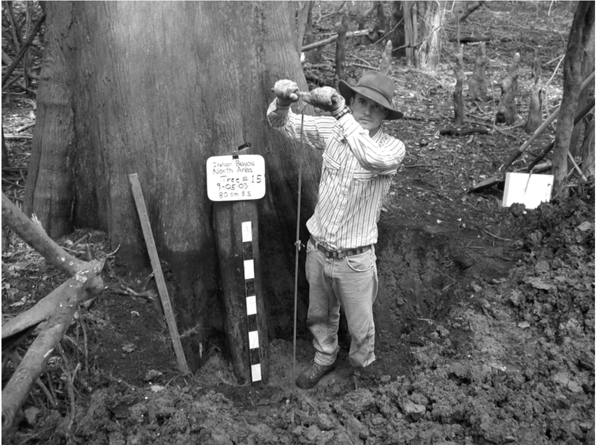
Figure 8-5. Field technician measuring cypress root depths with a 6-ft-long metal probe. View to the south. Date: 9/5/03.
