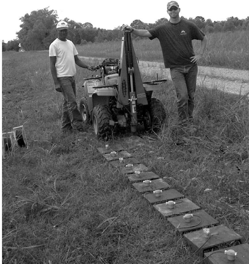
Figure 6-4. Flat-lying 12-in square aluminum plate (below vertical metallic bar) is struck by Accelerated Weight Drop (AWD) mounted on a four-wheel All-Terrain Vehicle. Data is collected both by geophones mounted on steel sleds and placed in the ground for comparison (Case 4). Date: 5/20/04.
