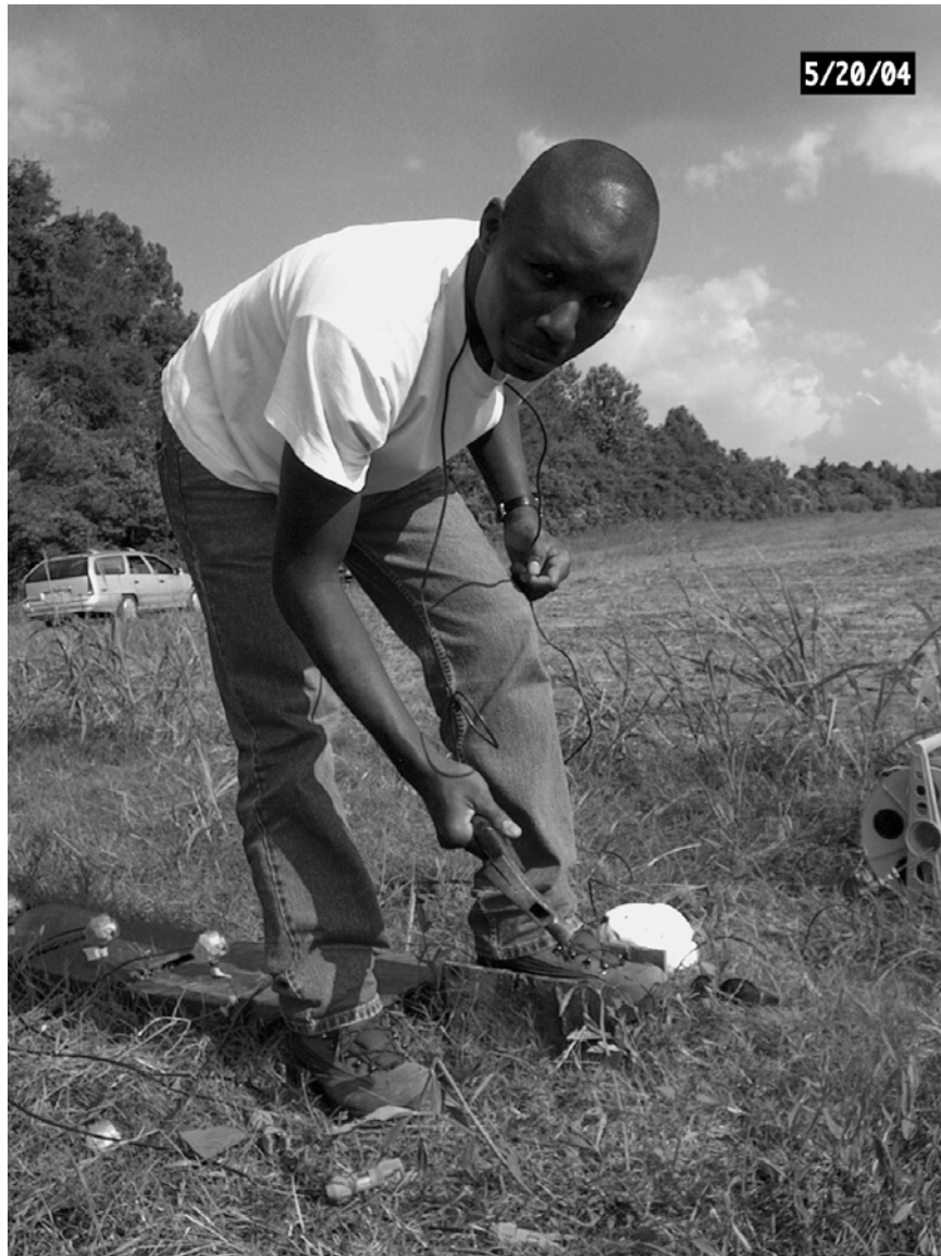
Figure 6-2. Steel I-beam struck by claw hammer. Shear phones in the ground and on steel platforms (Case 1). View to south. Date: 5/20/04.
