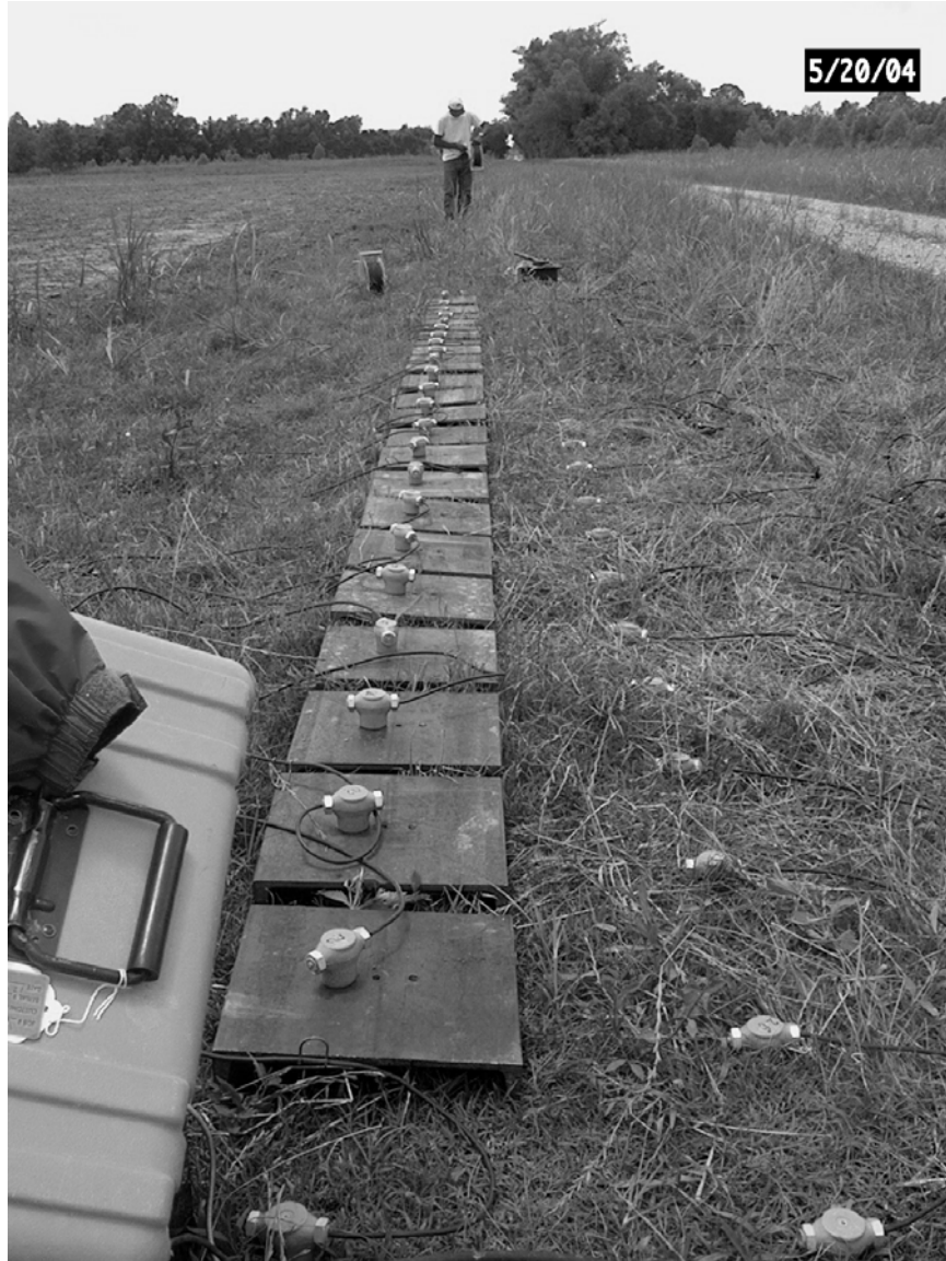
Figure 6-6. Twenty-three 100-Hz vertical geophone sensors are rigidly attached to C-channel, soft steel platforms plus one in the ground. Each sled weighs ~20 lbs. and is 10 in. long. The heavy weight assures suitable mechanical coupling with ground. The seismic source was generated by (1) a claw hammer (Case 2), (2) the impact of an AWD on a 12-in square aluminum plate (Case 4). This line of geophones is oriented from west (farthest point) to east). Geophones are placed one foot apart. This site is adjacent to Auger A-10 and Core C-5. Date:
