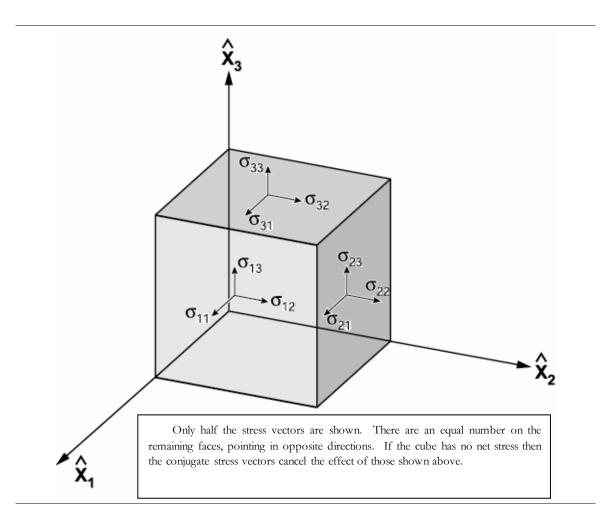
Each face of the cube can experience traction or stress. We take as convention that the surface stress acts on the outer surfaces of the cube upon the inner surface. Stress on a surface can be treated as a "stress vector" and is also called a **traction vector**  $(\vec{T})$ , where, in the limit, traction equals force per unit area at a point on one face in the direction normal to the face  $(\hat{n})$ :
