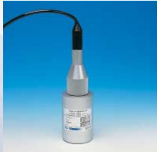
The L-4 is an INSTRUMENT QUALITY 1 Hz or 2 Hz multi-purpose seismometer that is small, light, and economical. It is designed specifically for scientific studies, yet has the ruggedness required for petroleum exploration work.
