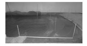
Figure 1. Louisiana State University seismic physical modeling sand tank (Figure 1)
