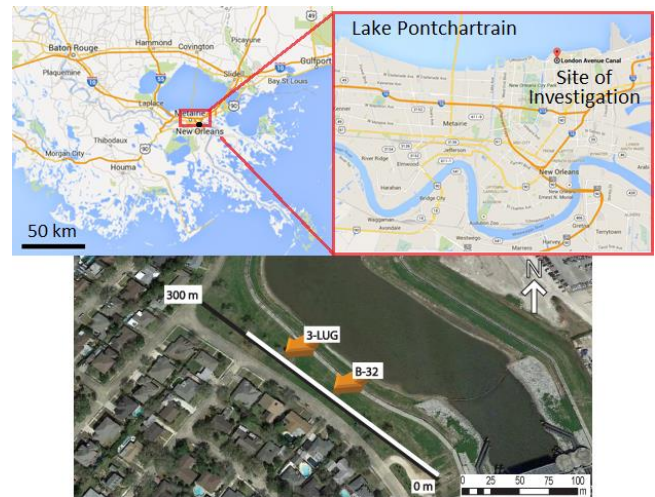
Figure 1: (Top) Site of investigation is the London Avenue Canal levee in London Park, New Orleans, LA. (Bottom) The long black line marks the location along which we derive resistivity (Figure 5), and shorter white line marks the length of the seismic profile (Figure 7). The locations of the boring logs, B-32 and 3-LUG, are marked with arrows at 128 and 159 meters, respectively, along the profile.
